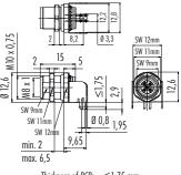
Thickness of PCB: ≤1,75 mm Hexagon nut enclosed loose
