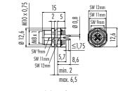
Thickness of PCB:  $\leq 1,75$  mm Hexagon nut enclosed loose
