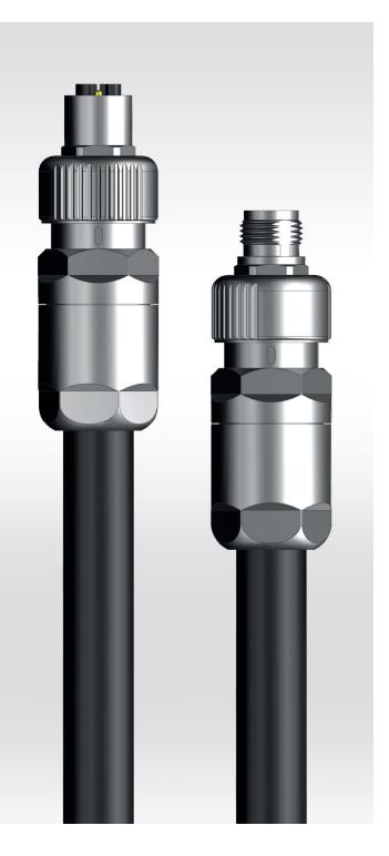
The PROVERTHA M12 Power connectors with L-Codierung 4+ PE are standardized in the IEC 61076-4-111. The PROVERTHA M12 Power connectors characterised by a full metal housing and the vibration-proof crimp techology for the power contacts. The connectors are designed for a wide cable clamping range für cables with wire sizes up to 2,5 qmm and outer diameters up to 14 mm. The connectors are the right solution for applications with
